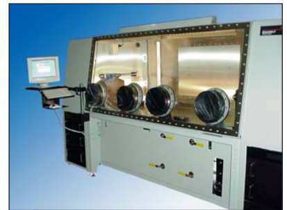
NOVA-CA and NOVA-G3 controlled atmosphere laser welding workstations for demanding applications in the medical and aerospace and defense electronics industries
