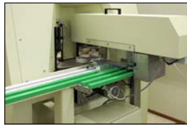
A pick and place robot is loading and unloading parts into the NOVA-T.
