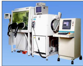
NOVA-CA and NOVA-G3 controlled atmosphere laser welding workstations for demanding applications in the medical and aerospace and defense electronics industries
