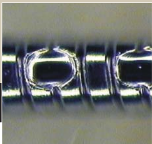
Laser Spot Weld, Hypo Tube
