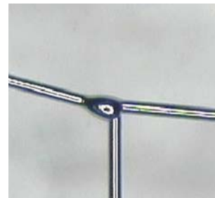
Resistance and Laser Spot Weld, Wire Joining
