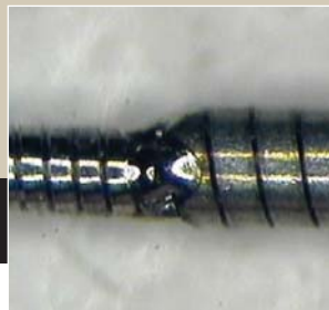
Laser Spot Weld, Hypo Tube
