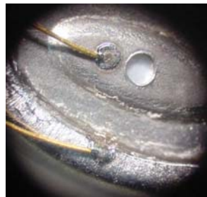
Resistance Spot Weld, Hearing Aid Wires
