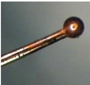
Resistance Spot Weld, Thermocouple Joining
