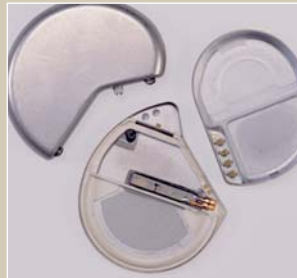
Resistance Spot Weld, Pacemaker Interconnects
