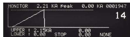
Monitor Screen – Shows weld current exceeding limit.
