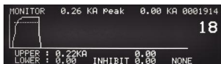
Monitor Screen – Shows 1st Pulse weld current exceeded limit.
